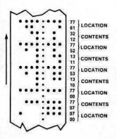
RIM format tape uses pairs of adjacent columns to represent 12-bit binary words directly. Channels 1 through 6 are used to represent either addresses or information to be stored. A channel 7 punch indicates that the current column and the following column are to be interpreted as an address specifying the location at which the information contained in the following two columns is to be stored. The tape leader and trailer for RIM format tape must be punched in channel 8 only (octal 200).
