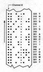
The USA Standard Code for Information Interchange (ASCII) format uses all eight channels¹ of the paper tape to represent a single character (letter, number or symbol) as shown in the diagram at left.
